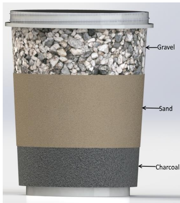
Figure 2. Design of filtering column
