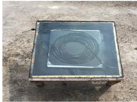
Fig. 1.2 Constructed Solar Water Heater
