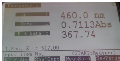
Fig. 10: Absorbance of methyl Orange solution where activated carbon was soaked which is activated by 50% Calcium Chloride Solution
