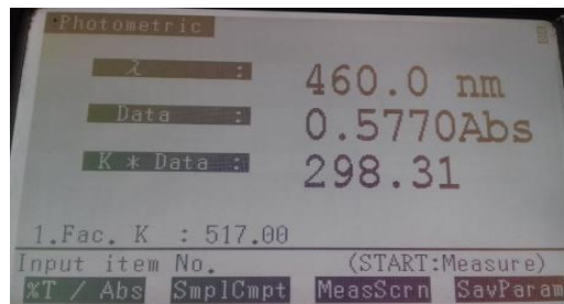
Fig. 8: Absorbance of methyl Orange solution where activated carbon was soaked which is activated by 50% Sodium Chloride Solution
