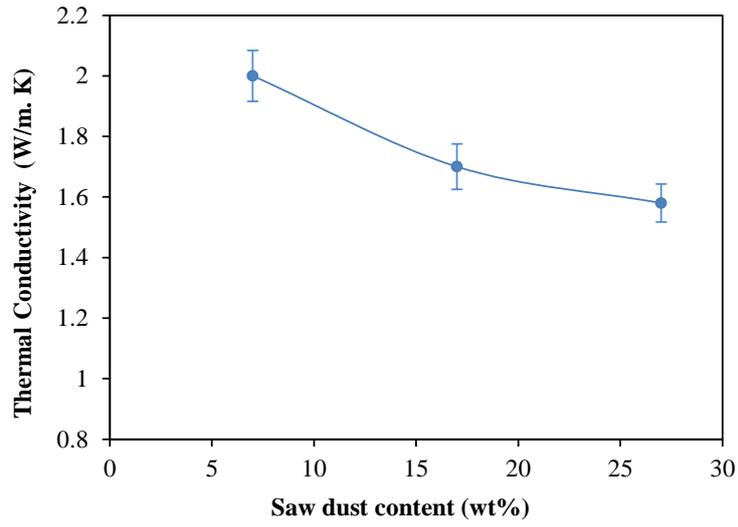
Fig.2 : Effect of saw dust on thermal conductivity
