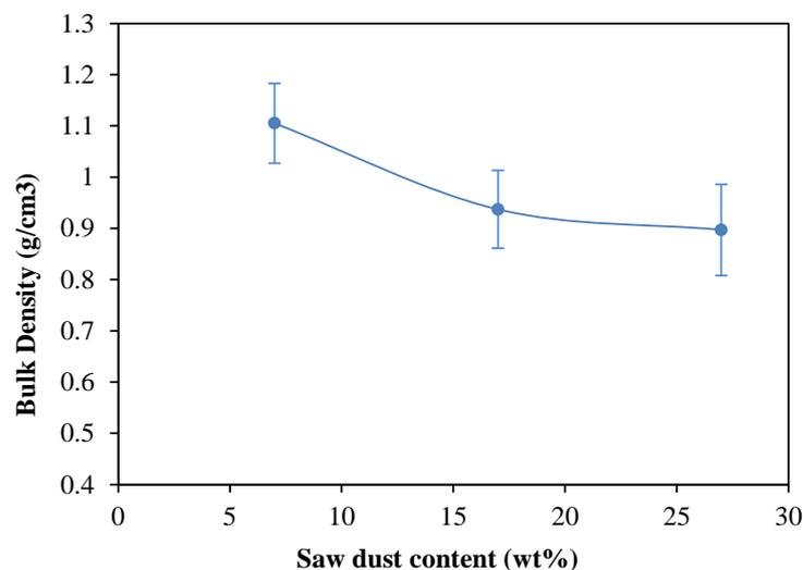
Fig. 1: Effect of saw dust on density
