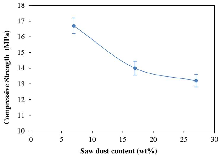
Fig.3 : Effect of saw dust on compressive strength.
