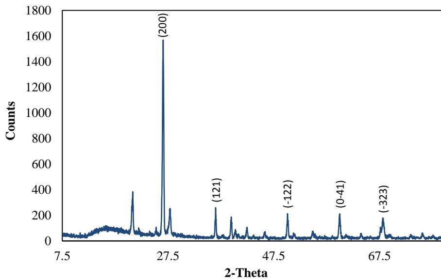
Fig.4 : XRD Analysis of Refractory insulating brick.
