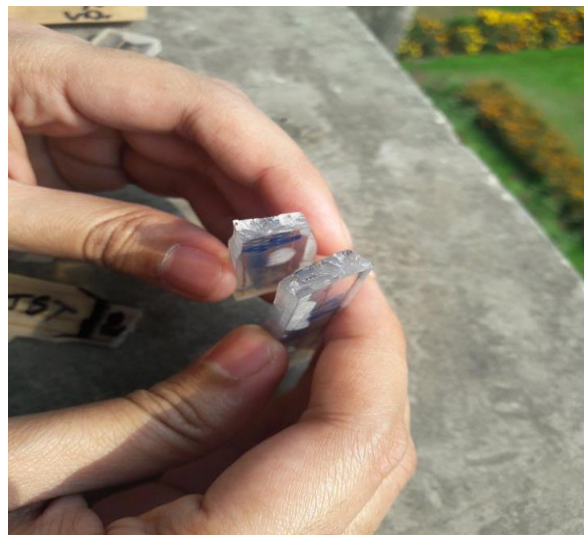
Figure 6: Fracture surface of the composite
