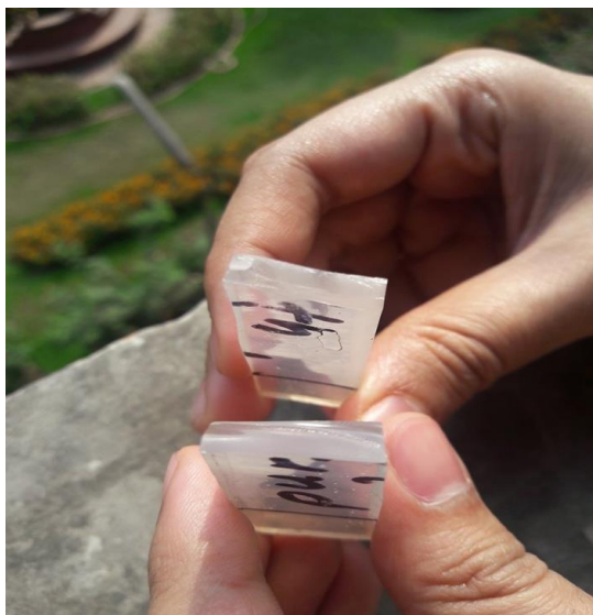
Figure 5: Fracture surface of pure polyester casting
