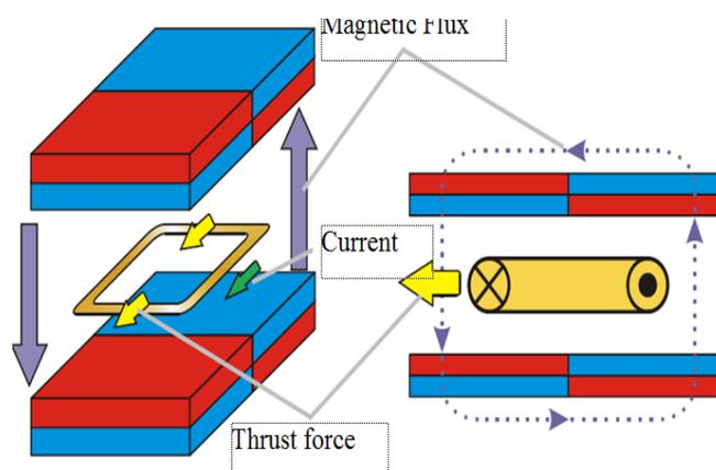
**Fig.2.** Working principle of VCM
