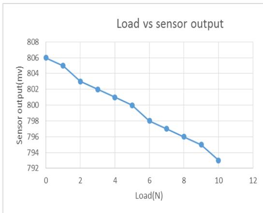
Fig. 5 Load vs sensor output
