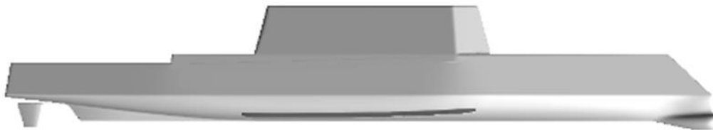
Fig 1. Geometry model of ONR Tumblehome (from Tokyo 2015 CFD Workshop)
