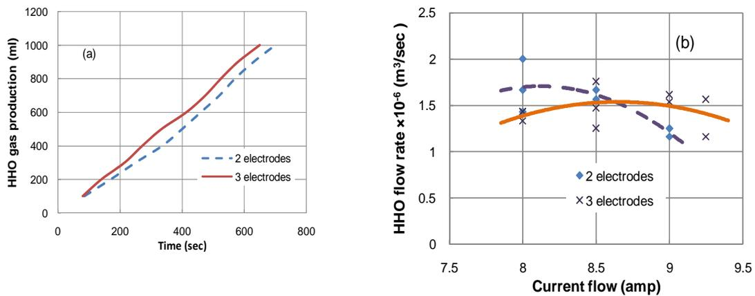
**Fig.4.** (a) HHO gas production (in ml) as a function of time and (b) HHO gas production rate (in m<sup>3</sup>/s) as a function of current flow for 0.5% KOH solution.
