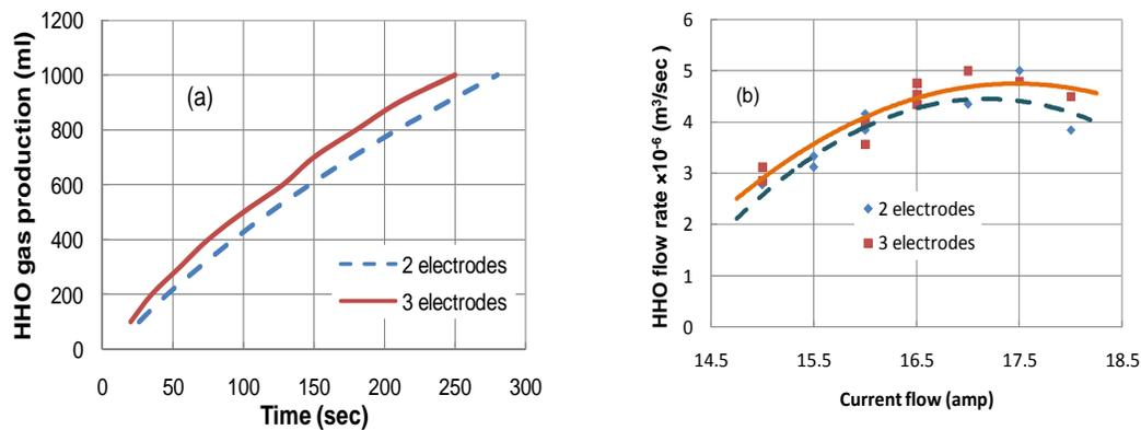
**Fig.5.** (a) HHO gas production (in ml) as a function of time and (b) HHO gas production rate (in m<sup>3</sup>/s) as a function of current flow for 1.0% KOH solution.
