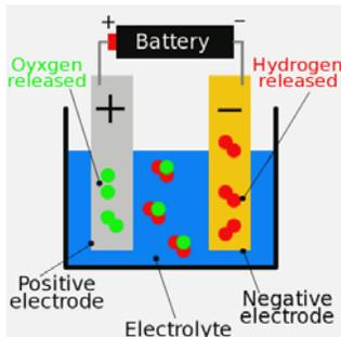
Fig. 1. Alkaline Electrolysis [14]
