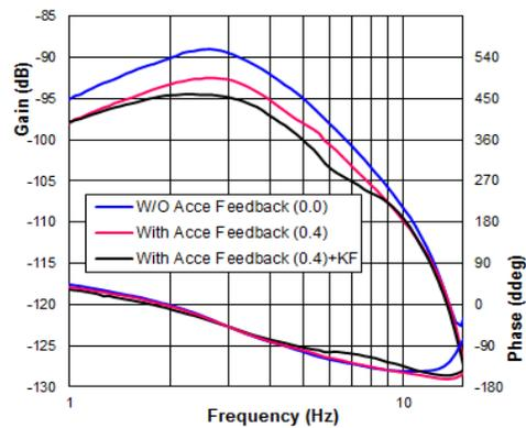
**Fig. 10** Effect of KF estimated acceleration feedback
