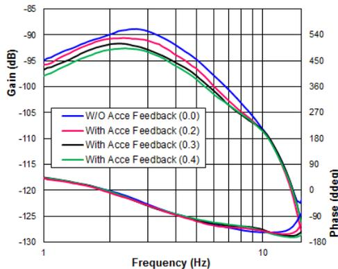
**Fig. 9** Frequency responses for different acceleration feedback gain
