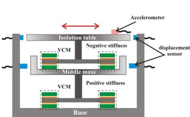
Fig. 2 Structure of horizontal vibration isolation system
