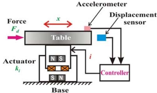
Fig. 4 Basic model of single axis control system
