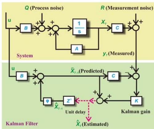
Fig. 6 KF algorithm by block diagram
