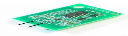
**Fig. 4.** HSM-20G Humidity Sensor
