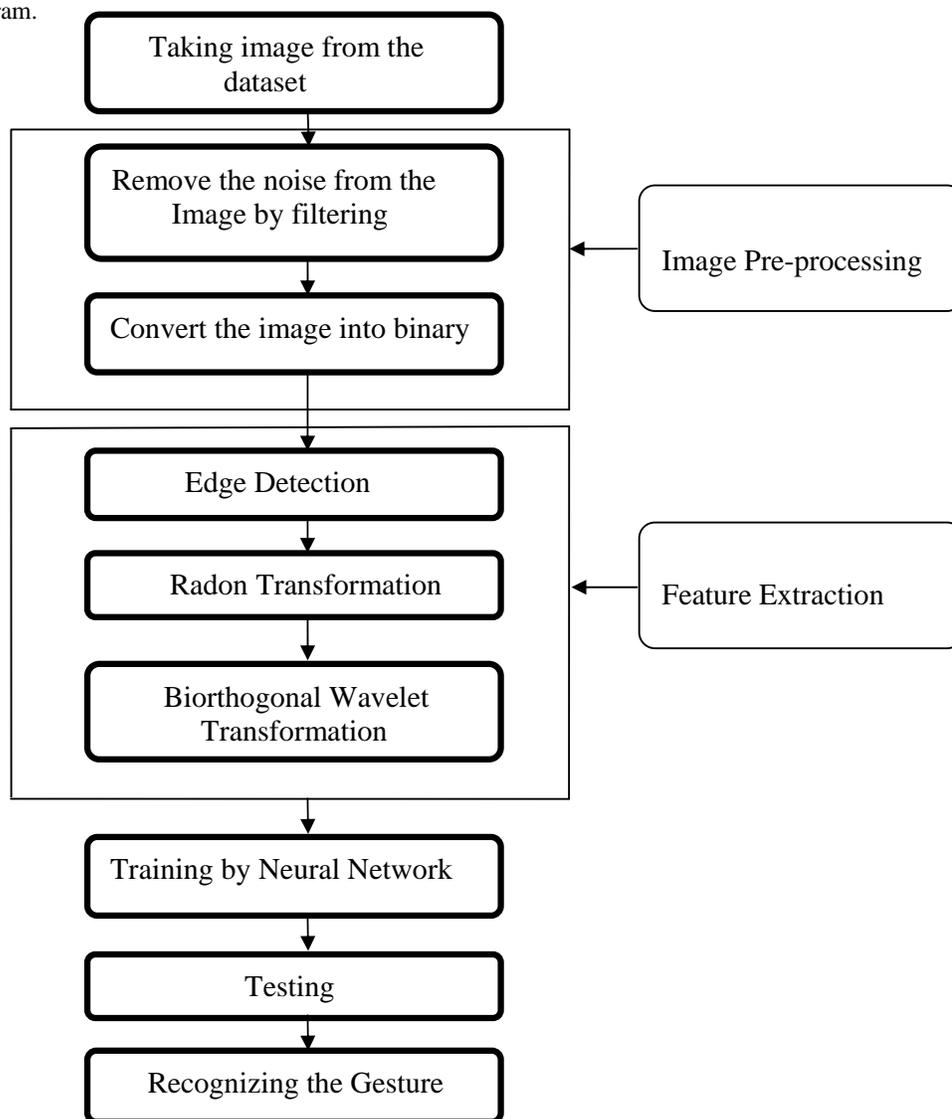
Fig.3. Block diagram of Hand Gesture Recognition System
