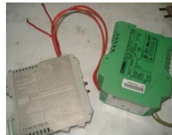
(C) Power supply unit
